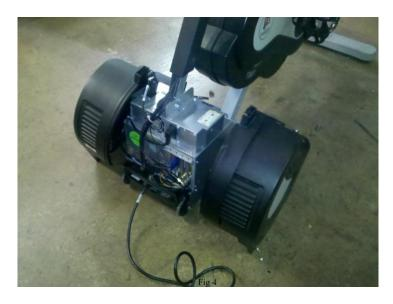
5) In the next step you will disconnect the cables that connect the computer to the bike. WE STRONGLY RECOMMEND TAKING PHOTOS AT THIS STEP BEFORE DISCONNECTING ANY CONNECTOR. This will make reconnecting your computer easier. There are connections on the front and rear of the computer. You may need to cut (USE EXTREME CAUTION) any wire ties to release the cables. (Fig 5 & 6)
