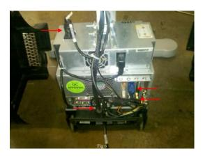
6) Your computer should now be free of the bike and can be packaged and sent in for repair. To reinstall the computer, simply reverse the above steps.
