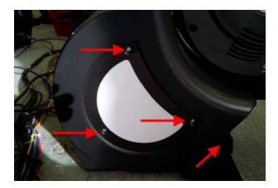
3) Remove the two center Phillips screws that secure the computer to the bike computer tray.
